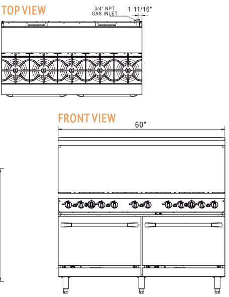
Keep combustibles a minimum of 17" away from the equipment. Keep a clearance of 4" at the rear.
