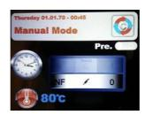
Confirm the selection touching again the icon Time or with the button. After that it is necessary to set the temperature that the probe will have to feel in order to stop the baking cycle.
