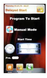
Modify the parameter "Hours" by touching the multi value scrolling set up icon and dragging the finger
