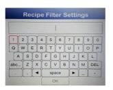
Digit the letters touching the corresponding button on the video, until composing the name of the desired recipe or part of the name. Press the icon confirm.
