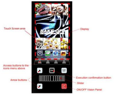
To interact with the interface, touch on the display the icon corresponding to the desired function.
