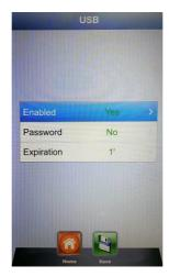
• Enabling: it allows to enable or disable the USB section in the Vision Full Touch control. Select the desired option dragging the finger towards right or left up to the desired value and confirm touching again the icon Alternatively use the slider to select the desired option and confirm with the button. In case the menu is disabled, the button disappears from the menus Chef and
